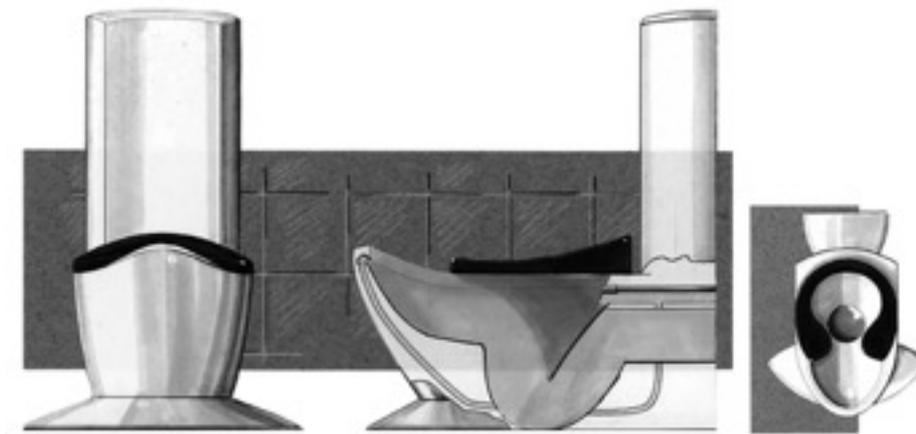
**Figure 6.** Materialized concept for lower point-supported toilet (front, side and top view) © Studio DenHartogMusch, Arnhem 1996.
